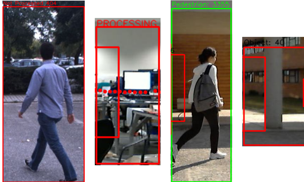
Figure 3.8: Different types of Candidate classifications, Not Processed (Unknown), Processing, Pedestrian, Object (Non-Pedestrian), left to right respectively.
