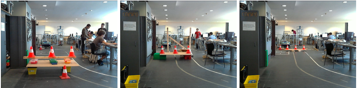
Figure 2.5: Manual Calibration Example: 3,8m / 6m / 10m from the LIDAR
